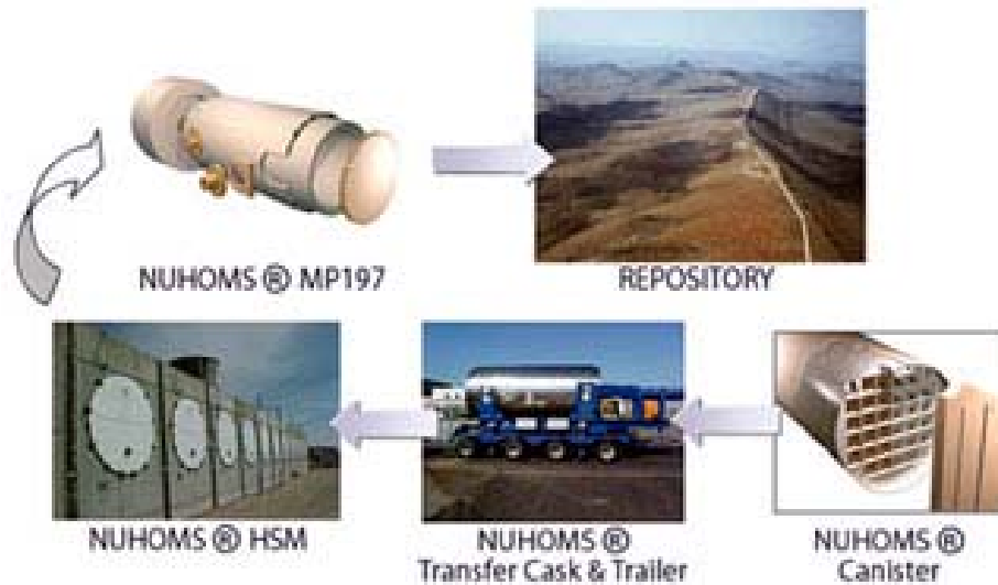
Figure G2-4. Transnuclear NUHOMS design (Note horizontal storage allowing stacking) (AREVA 2007).
