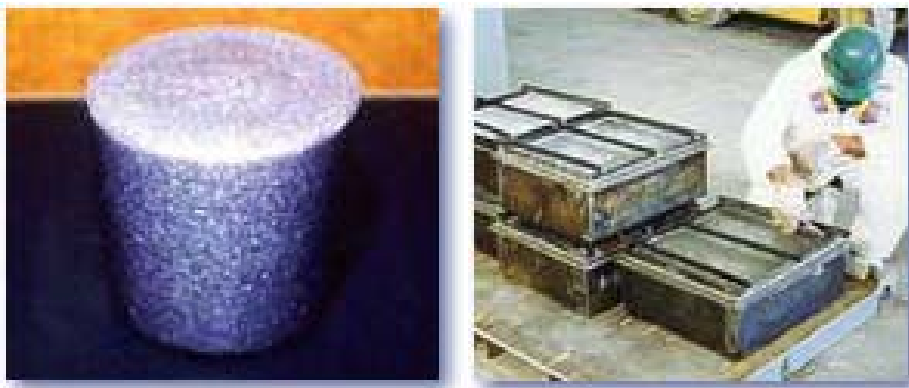
Figure G3-3. EnergySolutions microencapsulation and macroencapsulation of waste in plastic polymer. Figure taken from EnergySolutions Web site.
