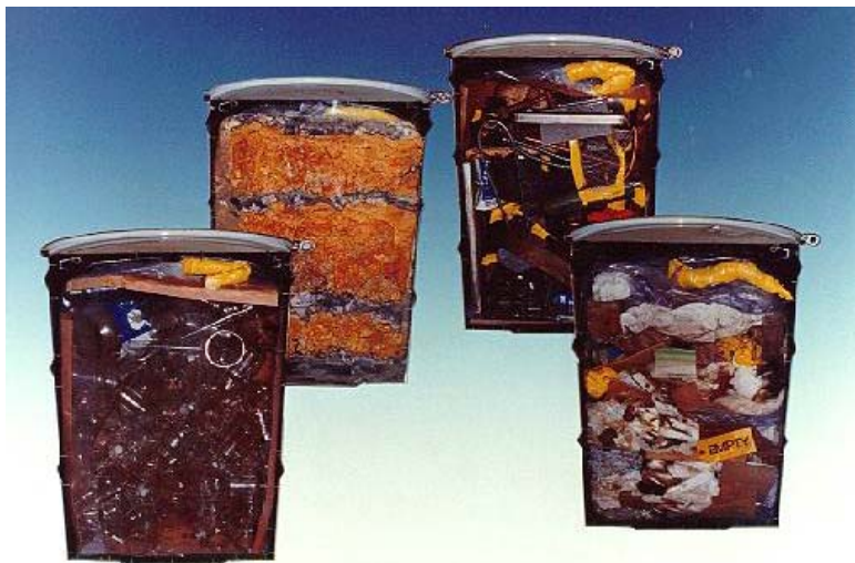
Figure G5-1. Legacy TRU wastes packaged in 55-gallon drums with and without liners, bags, and stabilizing sorbent media.
