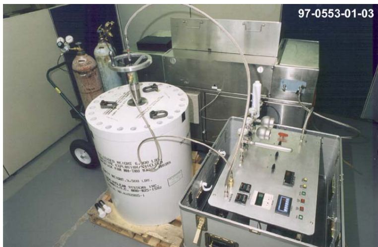
Figure G5-3. Headspace gas sampling of heated drum using Fourier transform infrared.
