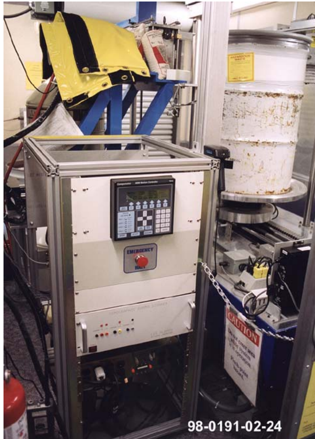
Figure G5-2. X-ray tomographic equipment for imaging drummed waste without opening the drum.
