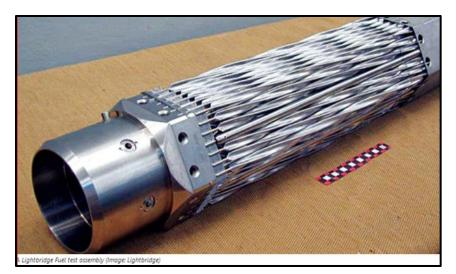
Figure D1-6A.8. A prototype Lightbridge/EnFission fuel assembly.
