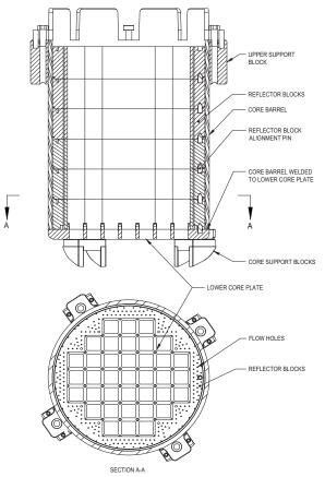
Figure A-10 VOYGR<sup>TM</sup> core supporting structure (NuScale 2020)
