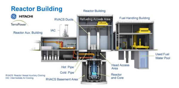
Figure A-4 General plant arrangement of Natrium (NRC 2022a)
