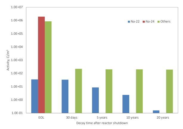
Figure 5-2 Coolant sodium activation and decay
