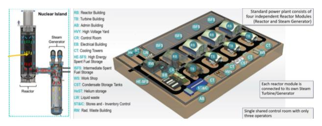
Figure A-5 Reactor module (left) and general plant arrangement of Xe-100 (right) (Courtesy of X-energy)
