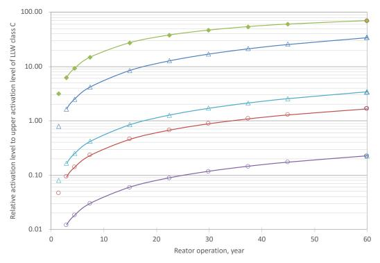
🔶 PWR-Baffle 🔶 SFR-Reflector 🔶 SFR-Baffle 🚣 Graphite block, 10 ppm 🚣 Graphite block, 100 ppm
