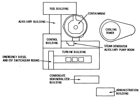
Figure A-2 General plant arrangement of reference PWR (Smith et al. 1978)
