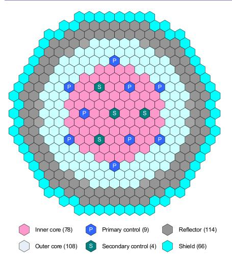
Figure 3-1 840 MWt core configuration used for Natrium waste assessment
