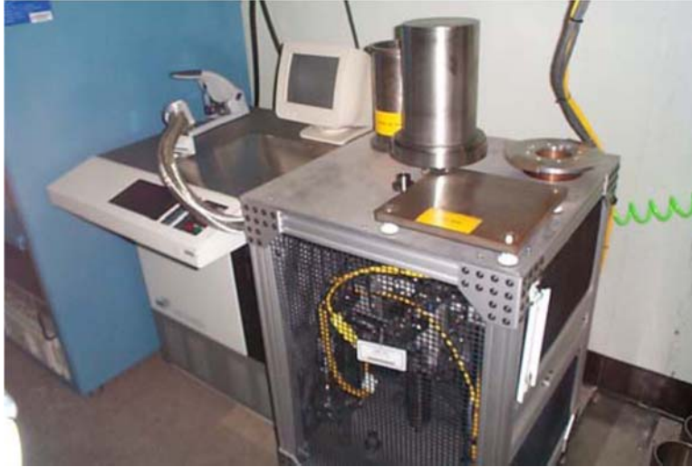
Figure E3-6. Test of leak detector installed in FB-Line Facility at SRS (Hudlow 2004).
