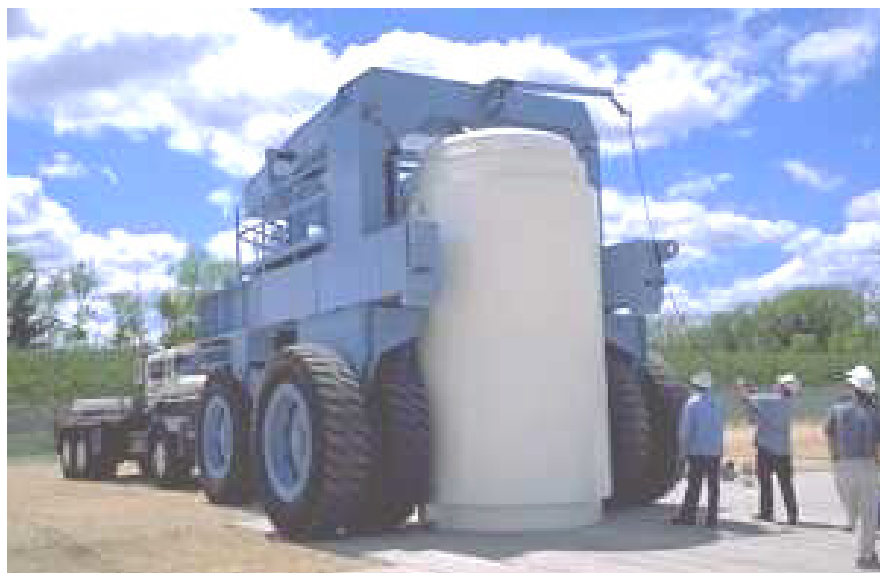
Figure E2-7. Dry storage cask transporter.
