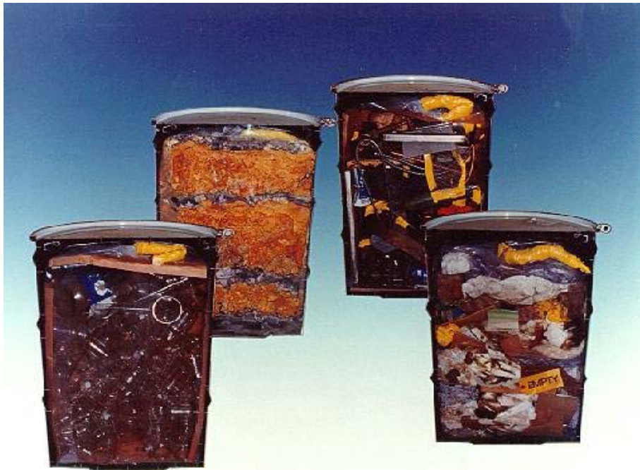
Figure G-13. Legacy TRU wastes packaged in 55-gallon drums with and without liners, bags, and stabilizing sorbent media.
