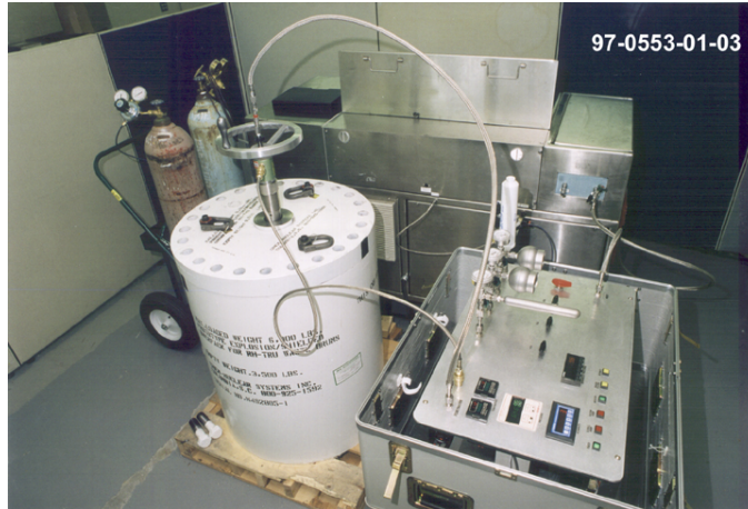
Figure G-15. Headspace gas sampling of heated drum using Fourier transform infrared.
