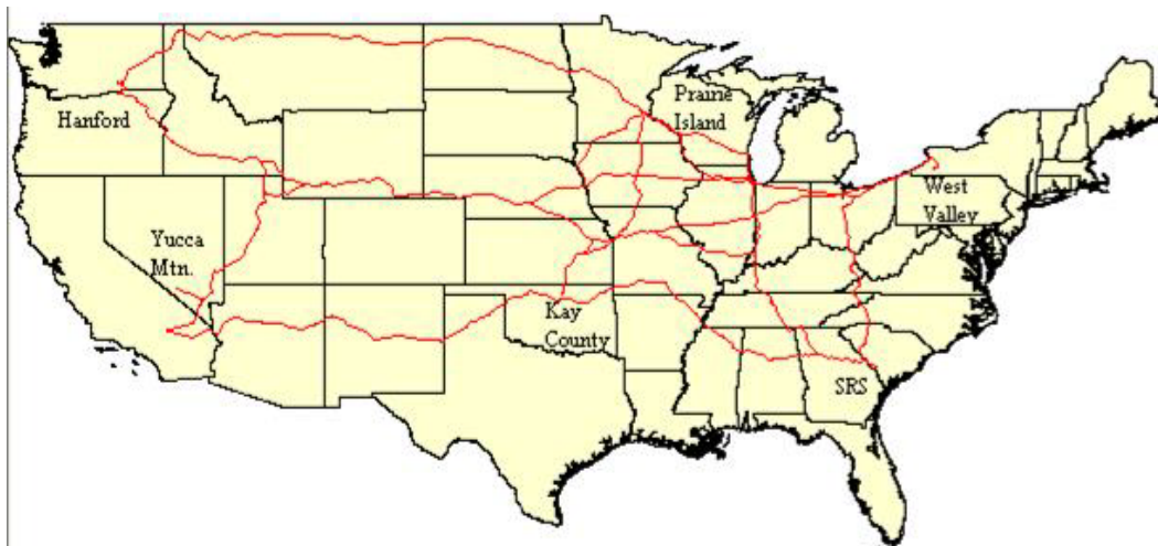
Figure OX-3. Mainline rail routes calculated using TRAGIS that connect the six hypothetical locations for regional facilities.
