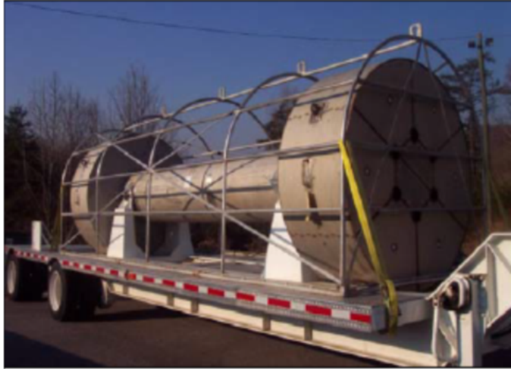
Figure 3. Transportation Configuration of the TN-FSV Cask (Turner and Lynn, 2004).
